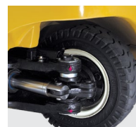
Extended steering axle for class leading manoeuvrability
