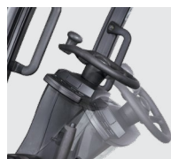
Infinitely adjustable steering column
