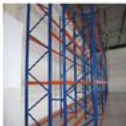
APR: Adjustable Pallet Racking – Double Deep LIFO High storage density, space utilisation increases. However, additional height clearances may be required. Suitable for low stock rotation or low throughput.
