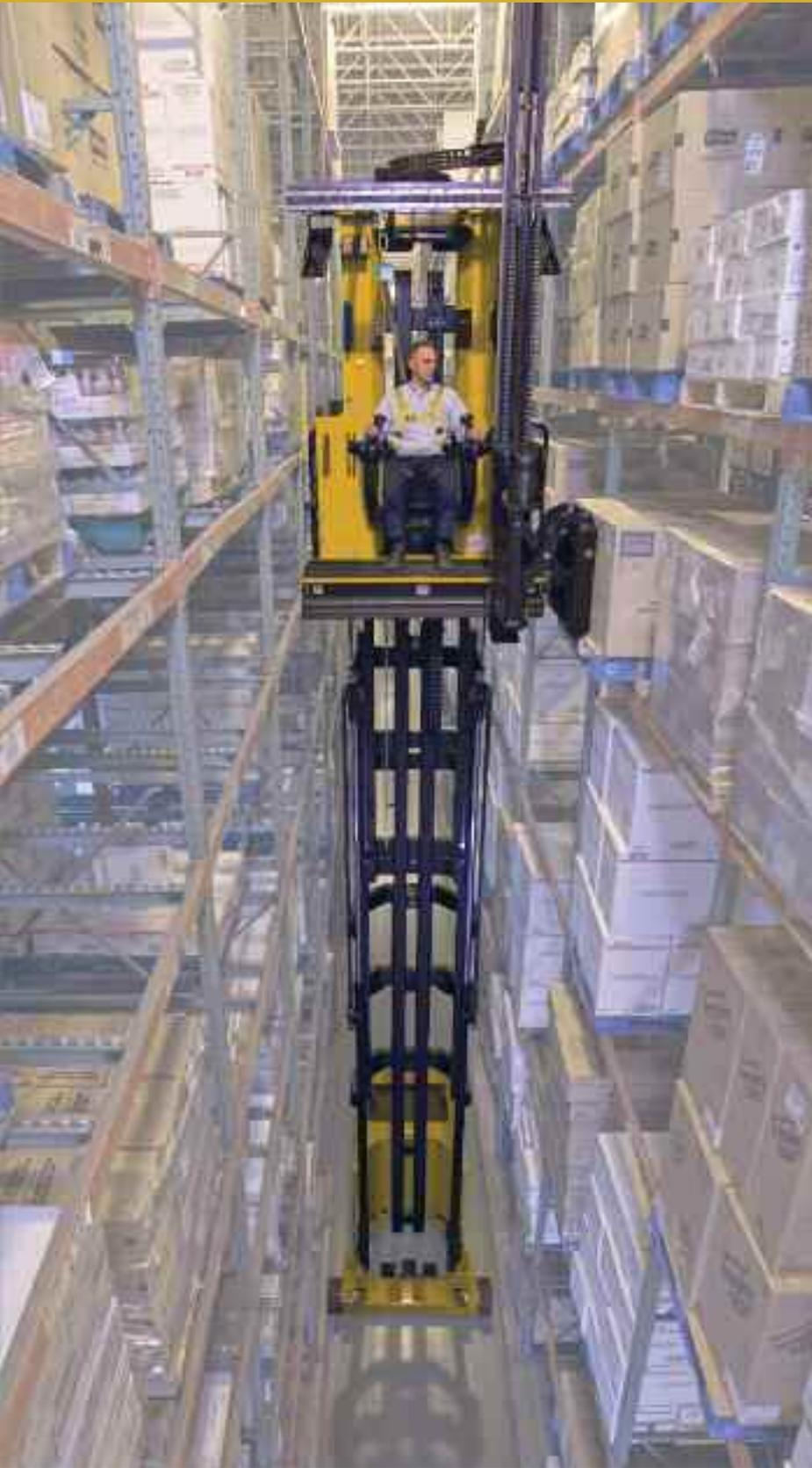
Available in 48 or 72 volts, **NTA-030SB** and **NTA-035SB** trucks are designed to meet and exceed your specific application requirements. **AC power** provides fast travel speeds, powerful acceleration and more responsive directional changes, increasing the number of loads moved per shift.
