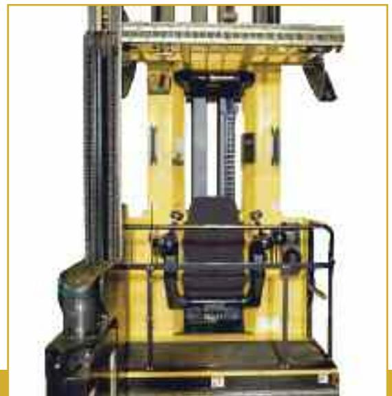
The spacious operator's compartment features **adjustable controls** and **infinitely variable armrests**, independent of the seat position. Intuitive seat-side controls are positioned for low effort operation, whether the operator is sitting or standing.
