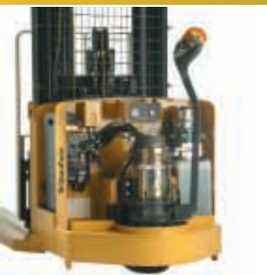
The MRW-E is designed for easy service access and maintenance. One power contactor reduces maintenance. The drive unit combines an integrated steer bearing and string guard to provide low maintenance and high up-time. The MRW-E comes standard with a low battery lift interrupt.
