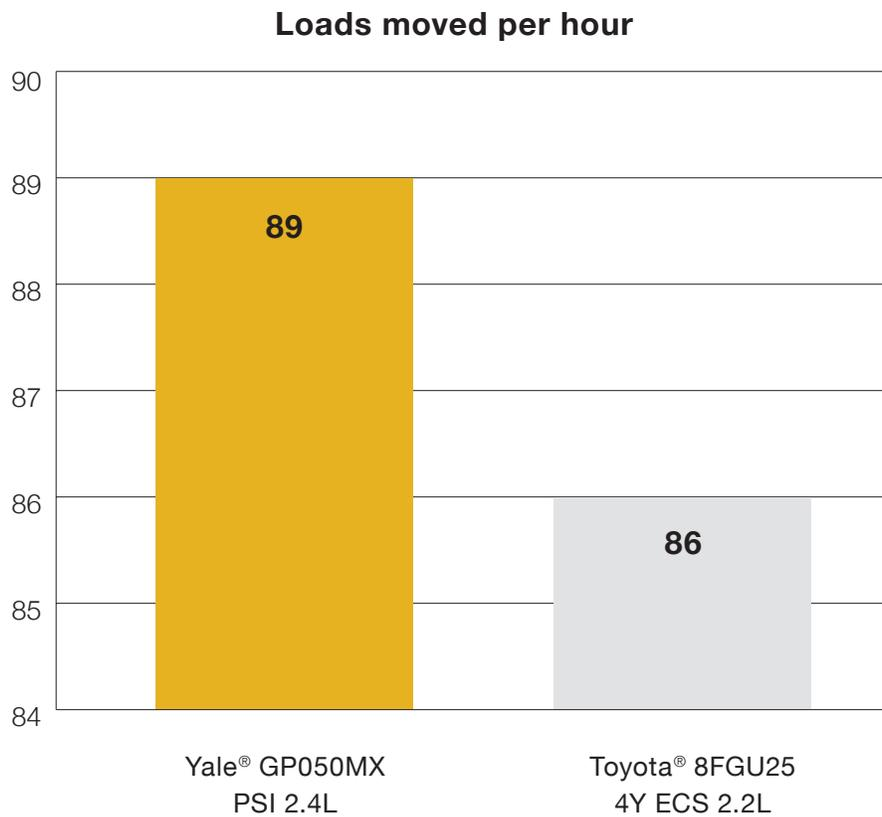
Three loads per hour adds up to major productivity over the course of a shift. Assuming the truck is in operation for seven hours, the Yale® GP050MX moves 21 more loads over the course of one shift and 63 more over three shifts. Considering a standard 48-foot trailer holds 24 pallets, the Yale MX enables operations to load nearly three more trailers over the course of three shifts.
