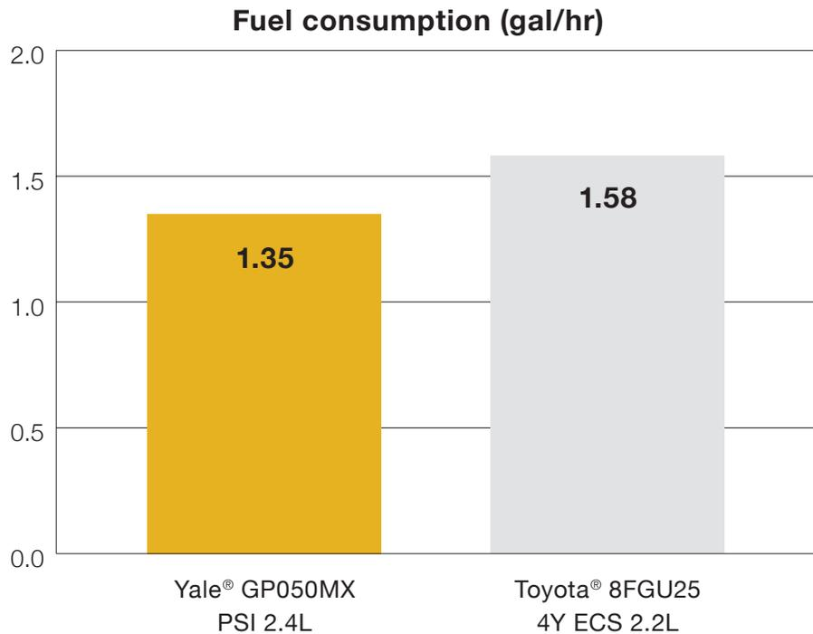
While 0.23 gallons per hour might sound small, it adds up to big savings over time. Assuming the truck works for seven hours out of an eight-hour shift, operations can save up to 1.84 gallons per shift. That equates to 5.52 gallons over a three-shift period, resulting in a financial savings of nearly \$15 at \$2.70 per gallon.
