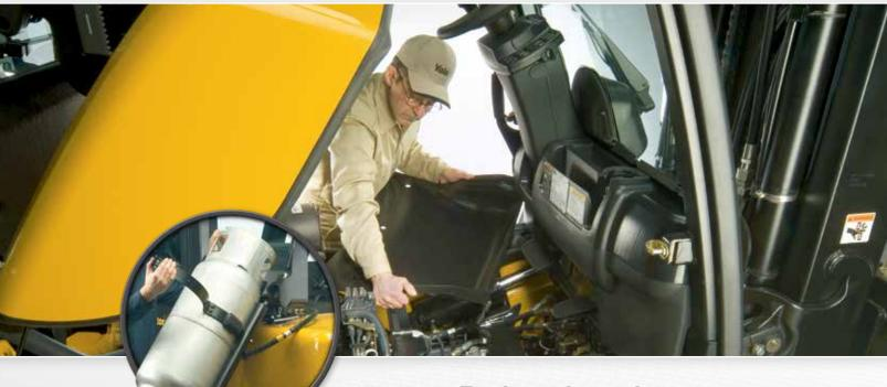
The optional swing-out, drop-down EZ-tank bracket swings out and drops down approximately 60 degrees for virtually effortless removal and installation of the LPG tank.
