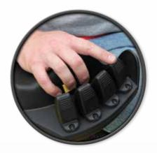
Optional Accutouch mini-lever electro-hydraulic controls
