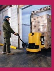
The Auto Deceleration System eliminates the need to manually apply a service brake for slow down. The operator simply returns the throttle control towards neutral for a controlled deceleration reducing fatigue and enhancing productivity.
