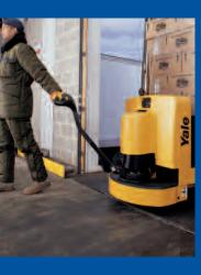
The bottom-mounted control handle design optimizes the operating position by increasing the walk behind clearance and reducing the steering effort.
