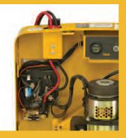
Simplified electrical system features a transistorized drive controller with integral hoist control that is easily programmed and features built-in diagnostics. Control handle serial communication reduces truck wiring and connectors decreasing the possibility of electrical problems. Hall effect sensor in the control handle eliminates high maintenance associated with potentiometers.
