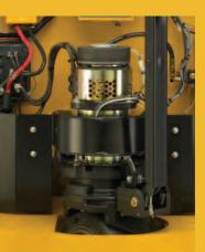
The use of an SEM traction system eliminates the need for directional contactors. The rigidlymounted traction motor design eliminates flexing and stretching of motor power cables. Drive unit features maintenance-free, permanently lubricated steer bearings. Electromechanical parking brake eliminates high maintenance associated with conventional drum and shoe brake. Standard string guard reduces the potential for drive axle bearing seal damage.
