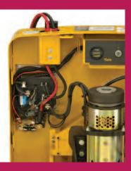
The electrical system has been designed using an advanced transistorized controller incorporating SEM technology to enhance truck performance and reliability. Each truck model uses a specifically sized traction motor with a controller programmed for that particular size motor. Further, your Yale technician can custom tailor the controller settings to meet the application requirements.
