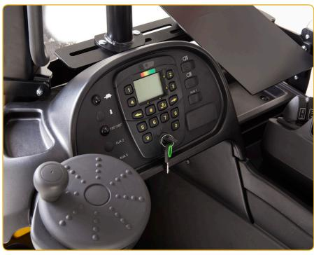
The steer positioning sensors provide feedback of the actual steer position. The standard steering has a 180° steer angle, a 360° option is available and enabled by the VCM software. A third option allows switching from 180° to 360° by pressing a steering mode selection switch on the dashboard. Speed reduction on cornering is automatic and can be adjusted.
