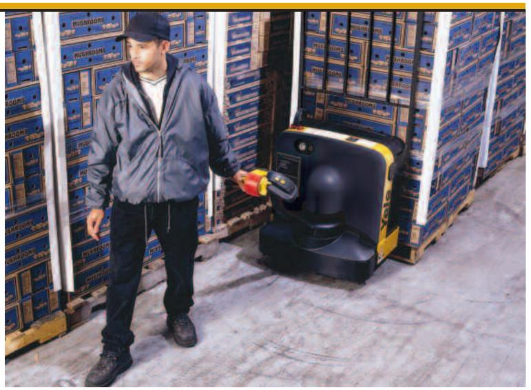
The ergonomically designed handle minimizes wrist movement and provides a solid grip for additional control while operating the unit. Lift, Lower, and Horn pushbuttons are conveniently located at the operator's fingertips. The butterfly throttle control provides multiple grip positions minimizing fatigue while allowing travel direction and speed to be selected by rotating the actuator in the desired direction of travel.
