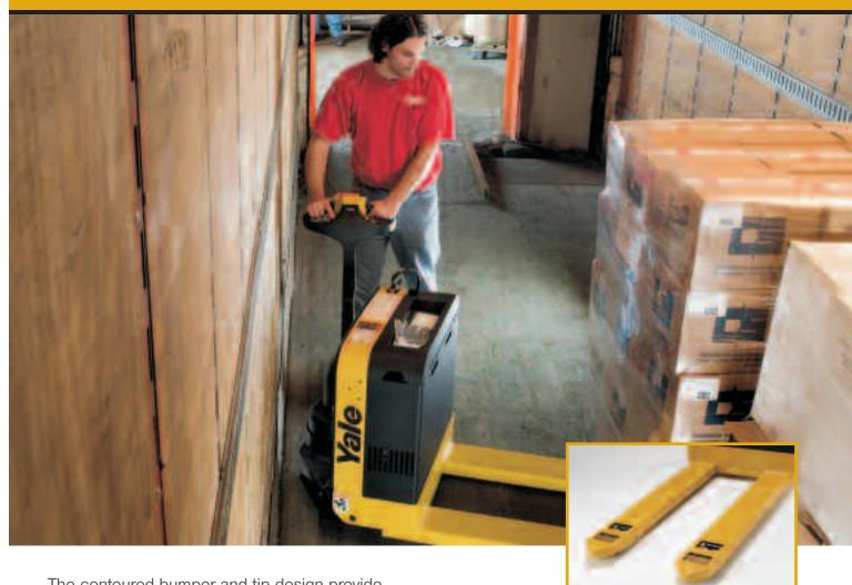
The contoured bumper and tip design provide industry leading maneuverability. The "Short E" option also includes a closed, tapered fork tip which improves angled pallet entry and exit, necessary when pinwheeling loads in trailers and during right angle stacking.
