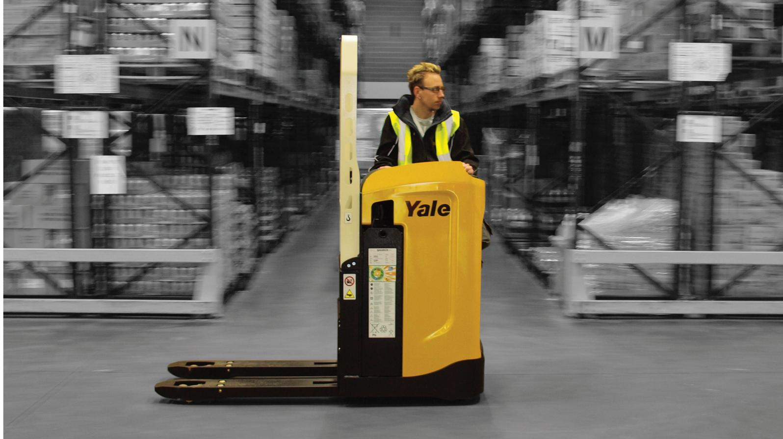
The MPT series of rider pallet trucks are designed with the operator at the heart of the manual handling function. Created to transfer goods over a range of distances while providing operators with a working environment that promotes fast cycle times and outstanding throughput levels, the sideways seat position offers excellent visibility in both travel directions while the adaptive seating allows the user to sit, lean or stand, offering maximum flexibility.
