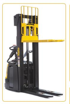
The adjustable pull rods give uniform lifting and lowering movement of the forks. The loading rollers are tandem with lubrication points and sealed bearings. Speed is automatically reduced with load arms raised.
