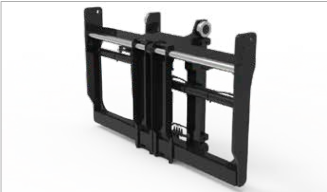
Pin type carriage with simultaneous and independent fork positioner.
