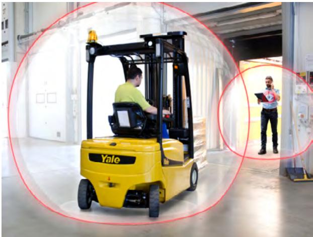
Operator assist solutions (OAS) are a step that warehouses can take today, speeding up dock-to-stock times by supporting both operator confidence and productivity. Disruptions like crashes or tip overs can delay product put away and result in equipment downtime that further hampers productivity. An OAS can help to limit the risk of these accidents by increasing reaction time and reinforcing adherence to best practices.
