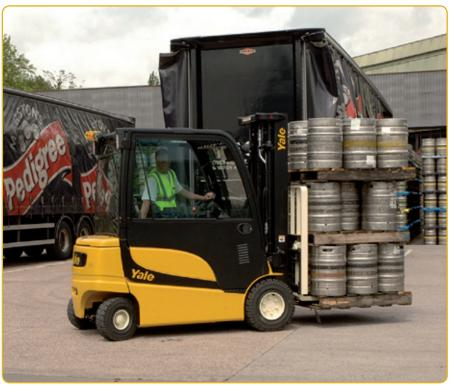
extended steer-axle that has increased articulation of the steer wheels, allowing it to turn in smaller spaces than a conventional 4- wheel steer-axle.
