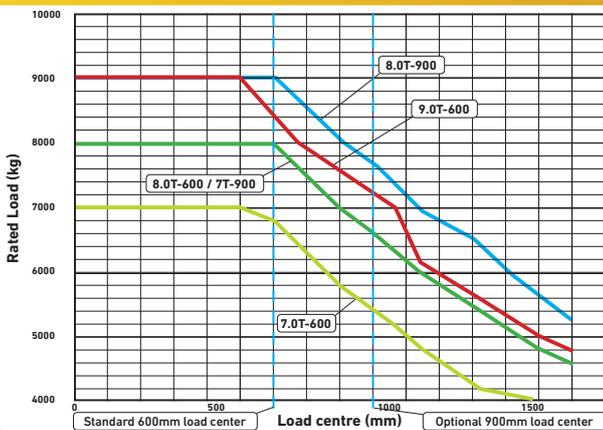
The ratings are computed using fork lengths as below:
