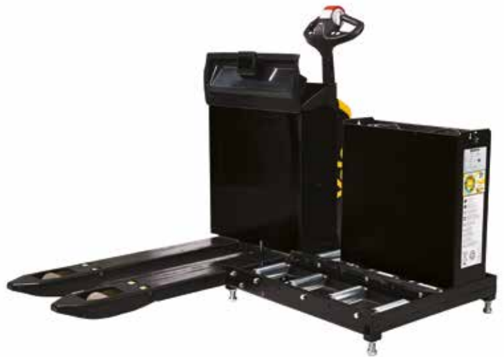
Battery side extraction available on MP 18-22 kg models.
