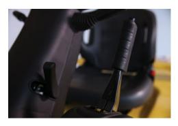
**HAND PARKING BRAKE**The low effort hand parking brake lever with button reduces operator fatigue.
