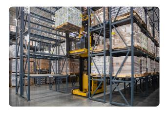
The <u>Yale very narrow aisle truck</u> won the business, emerging as the choice for both Unanue and Quinones. A major selling point was the tri-form mast, which offered industry leading support at all lift heights – including the maximum height of 55 feet – and visibility through the sides and center.
