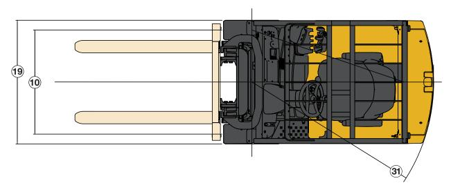
Circled truck dimensions correspond to the line numbers in the General Specifications chart. Dimensions are listed in inches (millimeters).
