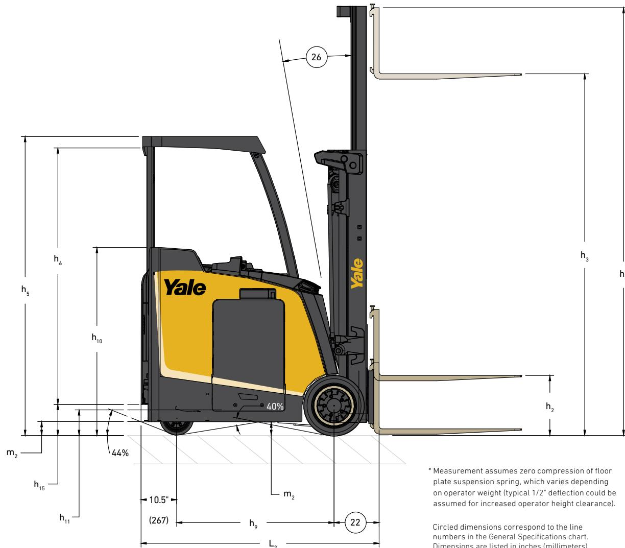
\* Measurement assumes zero compression of floor plate suspension spring, which varies depending on operator weight (typical 1/2" deflection could be assumed for increased operator height clearance).
