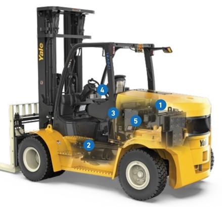
The Yale ERP-VNL series is the industry's first lineup of 15,500-19,000lb. counterbalanced lift trucks powered by an integrated, 350-volt lithium-ion battery. It was designed to satisfy a need for a zero-emission alternative in a high capacity range for both indoor and outdoor operation without sacrificing ICE-like performance.
