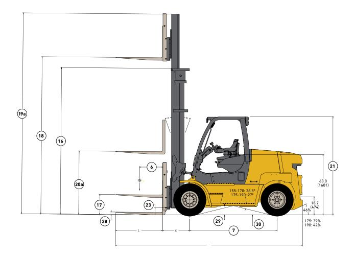
Circled truck dimensions correspond to the line numbers in the General Specifications chart. Dimensions are listed in inches (millimeters).
