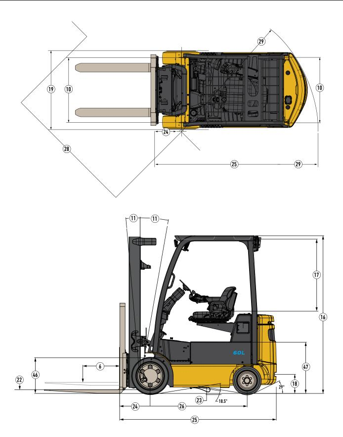
Circled truck dimensions correspond to the line numbers in the General Specifications chart. Dimensions are listed in inches (millimeters).
