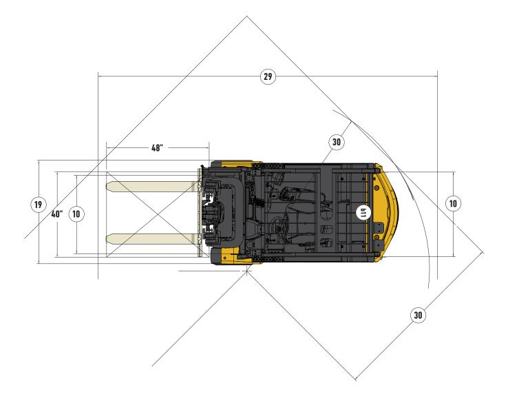
Circled dimensions correspond to the line numbers on the tabulated chart inside the spec sheet. Dimensions are in inches (millimeters).
