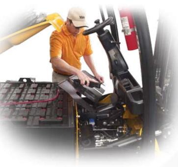
Lift-out floor plates require no tools for quick and easy service and checks. A rear-hinge hood offers exceptional access to components, making service easier.
