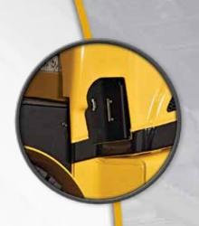
The multifunction display, located in the upper right corner of the operator's compartment, offers greater visibility for the operator with a large, LCD backlit screen for easy viewing and indicator icons for at-a-glance system status updates.
