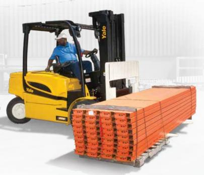
The "Zero Turn" radius steer axle and dual AC drive motors combine to provide extraordinary maneuverability in congested areas and narrow aisles.
