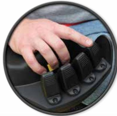
*Optional Accutouch mini-lever electro-hydraulic controls*
