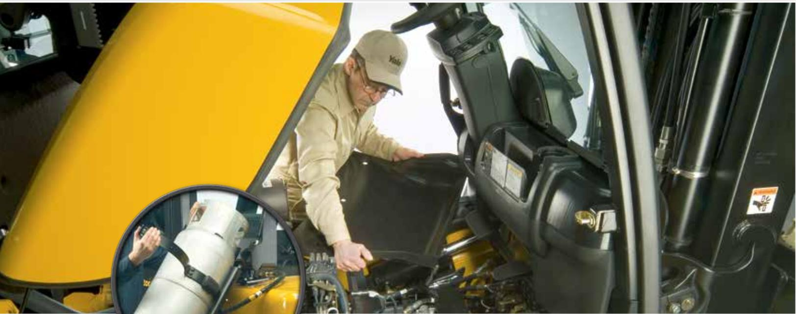
*The optional swing-out, drop-down EZ-tank bracket swings out and drops down approximately 60 degrees for virtually effortless removal and installation of the LPG tank.*
