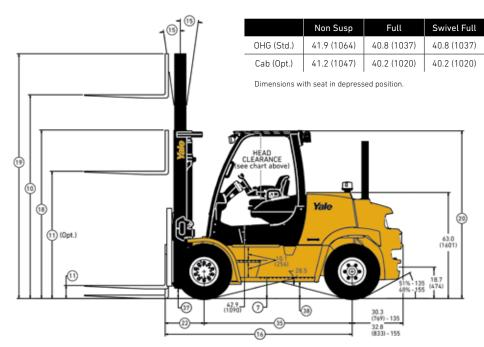
Circled truck dimensions correspond to the line numbers in the General Specifications chart. Dimensions are listed in inches (millimeters).
