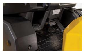
FOOTWELL DESIGN Familiar automotive-style pedal lay out contributes to ease of operation and load handling, helping to reduce operator fatigue.
