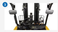
WIDE VIEW MASTS + A range of rigid 2-stage and 3-stage masts are available covering lift heights from 118"-256".
