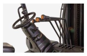
**COST-EFFECTIVE REPLACEMENT PARTS +** The grab handle with a horn button provides an ergonomic option during reverse travel, encouraging operators to look in the direction of travel while maintaining ability to sound the horn.
