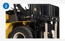
MULTIPLE CARRIAGE OPTIONS + Multiple carriage options, including side shifting and side shifting fork positioners for more precise load placement.
