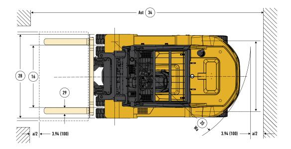
Circled dimensions correspond to the line numbers on the tabulated chart inside the spec sheet. Dimensions are in inches (millimeters).
