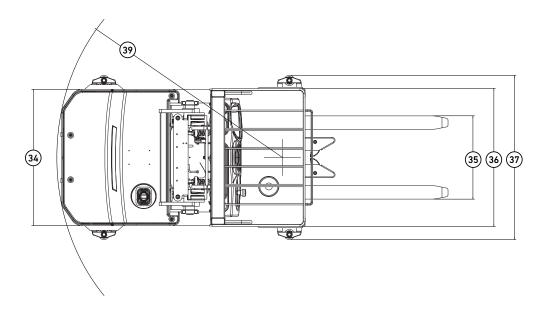
Circled truck dimensions correspond to the line numbers in the General Specifications chart. Dimensions are listed in inches (millimeters).
