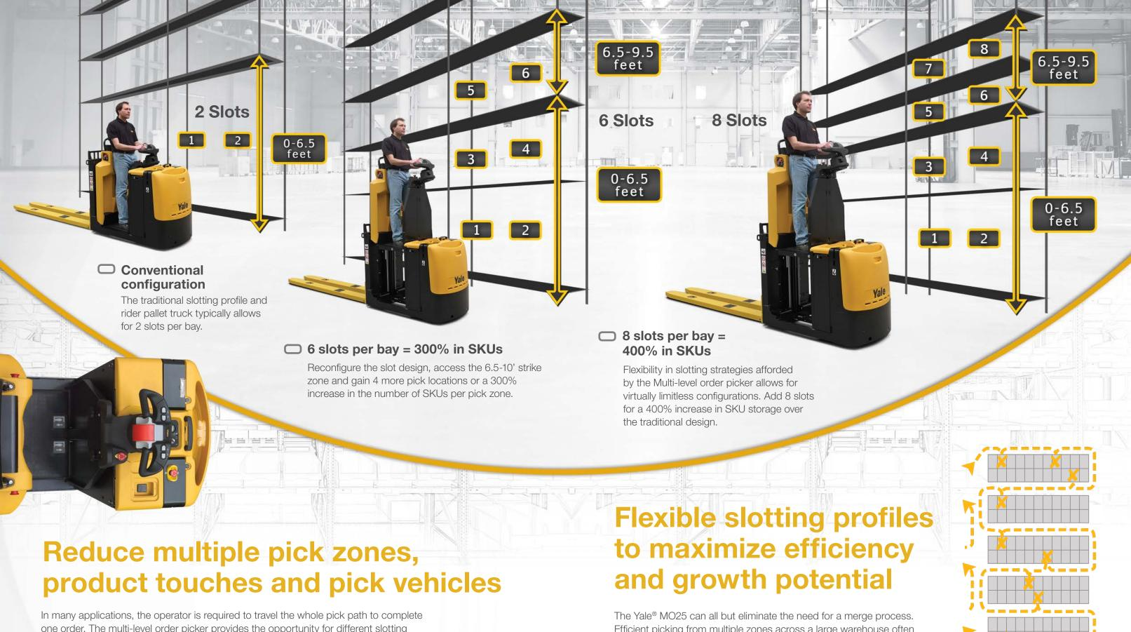
In many applications, the operator is required to travel the whole pick path to complete one order. The multi-level order picker provides the opportunity for different slotting strategies that will enable more SKUs to be stored in less space. Since the travel component of the pick process can make up to 70% of the total time, integrating the multi-level order picker into an efficient slotting technique can optimize the overall
