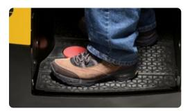
**OPERATOR PLATFORM** – The suspended floor system was engineered to rest on four (4) rubber isolators bolted to the drive frame to help reduce shock and vibration transmitted to the operator's feet, back and legs from dock plates, expansion joints and other irregular floor surfaces.
