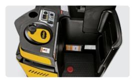
**OPERATOR COMPARTMENT** – An offset master drive unit (MDU) offers more usable floor space than a typical center-mounted model found on leading competitive trucks. This strategic, space-saving design combined with a contoured, urethane padding allows the operator to stand comfortably in a true side stance position and provides the flexibility to adjust stance throughout the shift.
