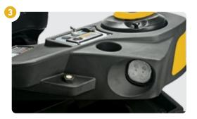
LED WORK LIGHTS W/ULTRASONIC SENSOR + - Help increase visibility and awareness in low-lit areas such as transport trailers with the optional automatic LED work lights<sup>4</sup>
