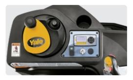
**POWER STEERING** – Fully adjustable (lockto-lock), electric power steering allows the operator to customize the steer effort to match personal preference and application needs. This feature may help build confidence and reduce fatigue in operators when maneuvering in tight, congested areas.
