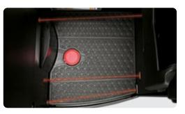
YALE® SMART OPERATOR SENSING SYSTEM <sup>(2)</sup> – The industry-exclusive, pedalfree design provides a comfortable, more intuitive working environment by eliminating the need for constant and restrictive foot engagement. This allows operators the freedom to adjust their stance and find a comfortable operating posture.
