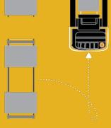
**180° STEERING** Truck has to come to a stop and direction of travel selected manually by operator.
