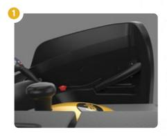
FORWARD STANCE WITH AFT TRAVEL CONTROL HANDLE AND AUTOMOTIVE STEERING ❖ — Natural steering familiarity in both directions can help shorten training time for new operators and may reduce facility and product damage
