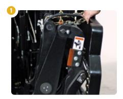
**PANTOGRAPH** can be disassembled in 4 steps to service or replace parts without removing the carrier from the mast
