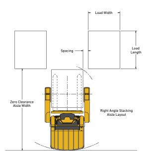
NOTE: These are "Zero Clearance" aisles and require an additional 6" to 12" to be added to provide for easier maneuvering.
