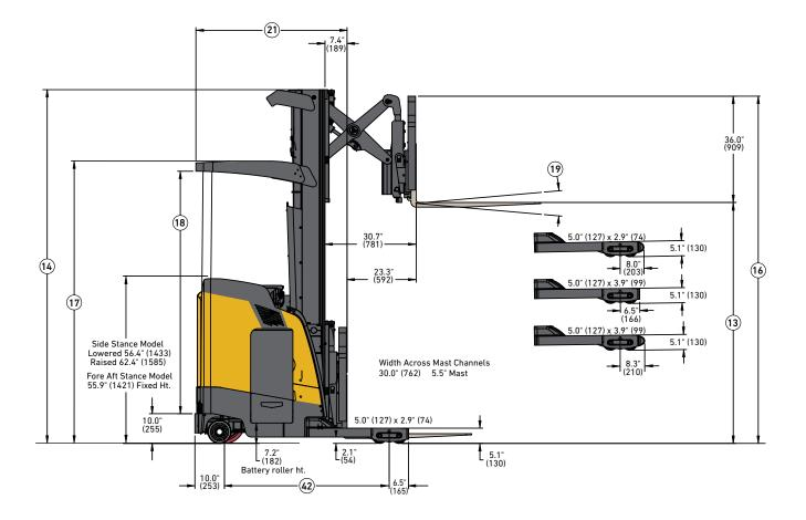
Circled truck dimensions correspond to the line numbers in the General Specifications chart. Dimensions are listed in inches (millimeters).
