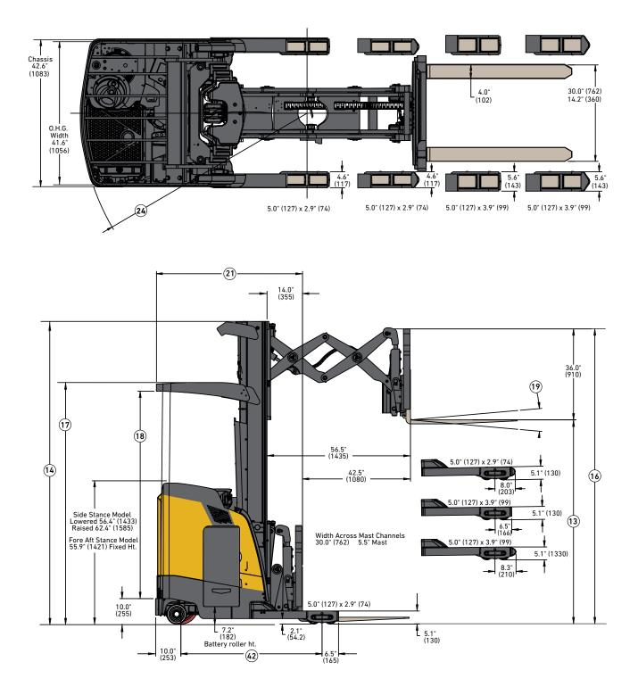
Circled truck dimensions correspond to the line numbers in the General Specifications chart. Dimensions are listed in inches (millimeters).
