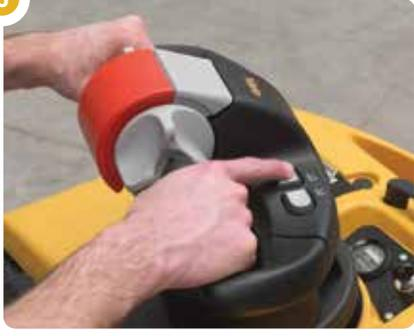
**POWER STEERING** – Fully adjustable, fly-by-wire power steering helps reduce steering effort by up to 90% by varying the amount of resistance based on the control handle position, steer tire angle and truck travel speed.
