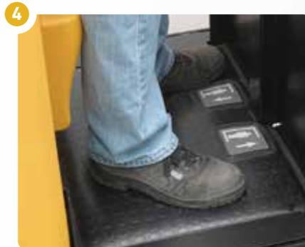
**4 OPERATOR PLATFORM –** The suspended platform helps increase operator comfort and allows easier pass through to optimize picking from both sides of the truck. The operator sensing floor mat covers the entire platform area to detect when the operator is on board. The optional lifting platform is foot controlled to facilitate ground and second level picking, reducing the distance the operator must reach when picking from rack to pallet.
