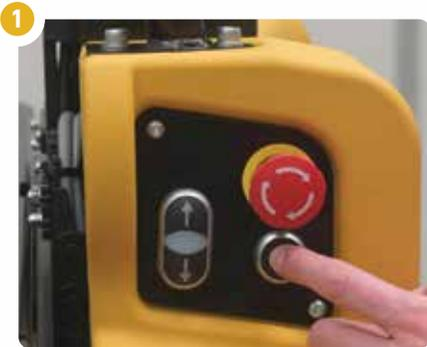
**1 COAST CONTROL –** Slow-speed forward and reverse buttons on both sides of the backrest allow the operator to advance the truck to the next location while walking alongside it. This eliminates the need for operators to climb back onto the truck, helping reduce fatigue and improve efficiency.
