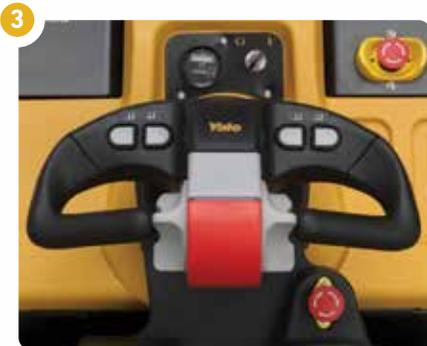
**3 CONTROL HANDLE–** Fingertip control reduces arm movement required to change direction, helping reduce fatigue and allows the operator to remain within the truck footprint at all times for protection. The wrap-around design keeps the operator's hands within the interior perimeter of the handle and the large control buttons are conveniently positioned to help reduce repetitive movement.
