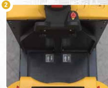
**2 OPERATOR COMPARTMENT –** The low step height of just 6 inches provides easy on/off access, while the floor compartment area accommodates large steel-toed boots. A high backrest that is soft to the touch and contoured, helping the operator locate the most comfortable operating position.
