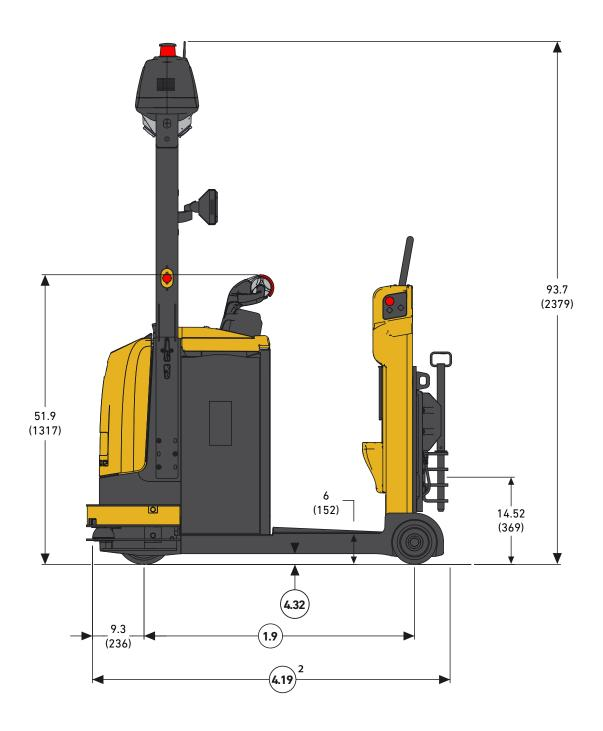
$Circled\ truck\ dimensions\ correspond\ to\ the\ line\ numbers\ in\ the\ General\ Specifications\ chart.\ Dimensions\ are\ listed\ in\ inches\ (millimeters).$
