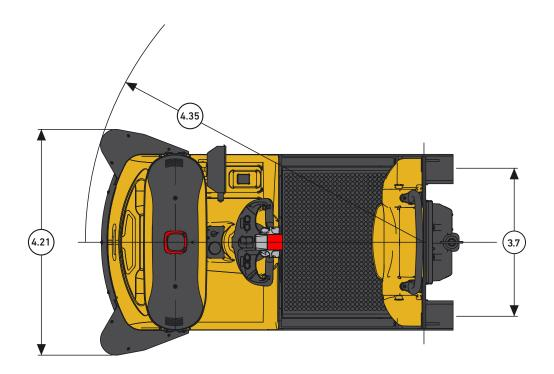
$Circled\ truck\ dimensions\ correspond\ to\ the\ line\ numbers\ in\ the\ General\ Specifications\ chart.\ Dimensions\ are\ listed\ in\ inches\ (millimeters).$
