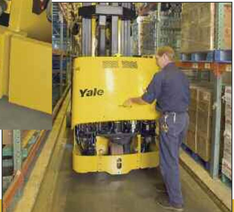
**Easy access** to all motors and controllers is provided through a one-piece hood with gas-assist lifting cylinders, conveniently located in the rear of the truck. Constructed of reinforced steel, the hood can be opened while the truck is in the aisle. Top battery access lid provides fast in-truck battery maintenance.
