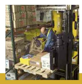
**Seat-side joystick controls** provide for simultaneous operation of truck functions. The operator can simultaneously control:
