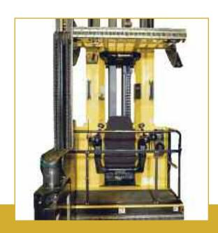
The spacious operator's compartment features **adjustable controls** and **infinitely variable armrests**, independent of the seat position. Intuitive seat-side controls are positioned for low effort operation, whether the operator is sitting or standing.
