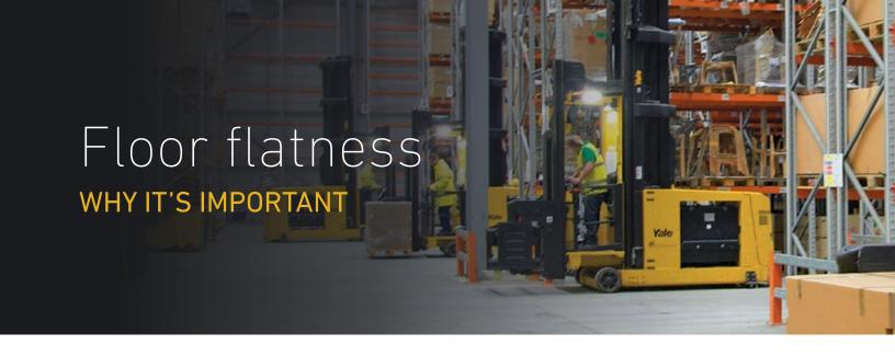
Flatness is an essential requirement of a floor slab in all categories of industry, none more so than in the aisles of high bay warehouses where defined path very narrow aisle (VNA) turret trucks operate. Even relatively minor variations in floor level between the wheel tracks of VNA trucks are magnified in direct proportion to the height of the racking they are operating within.
