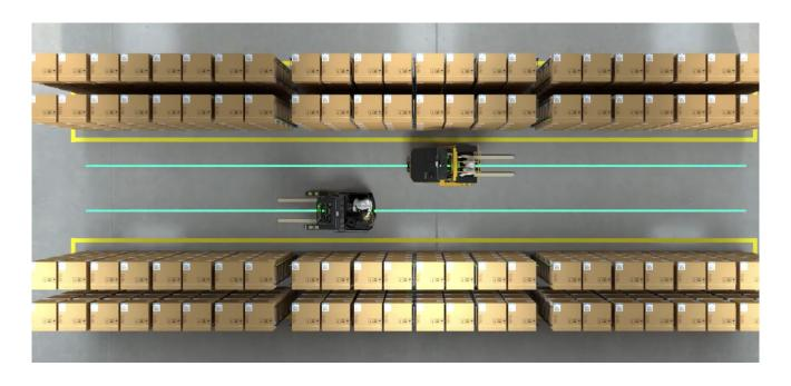
Object and pedestrian detection only work in the path of travel and if the object or pedestrian is standing straight up or vertically.
