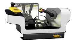
Using a simulator to sharpen skills may help reduce the risk of product damage, facility damage and injury associated with operating a real lift truck in an active work setting. This virtual approach allows new employees to practice in a safe, low pressure environment and helps them make the most of live, in-person training.
